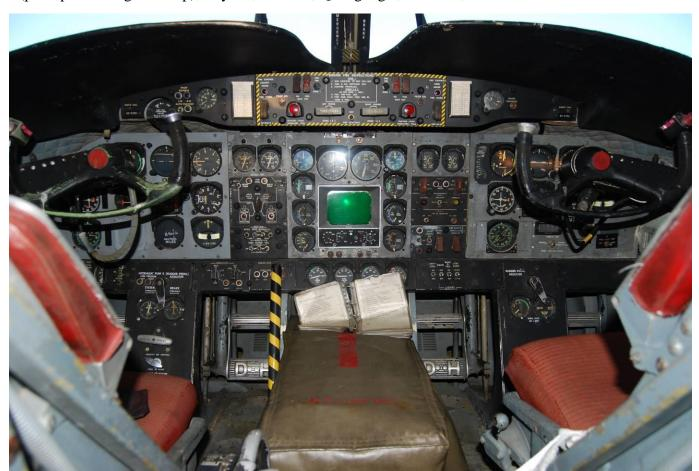
This photo shows the uncluttered instrument panel. The throttle quadrant was mounted overhead with the mixture and pitch controls. Also on the overhead console is the landing gear lever and just behind the engine controls is the aileron trim, ignition switches, flap control lever, and carburetor air-temperature control lever.
