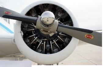
radial engines, each developing 450 horsepower. Nothing sounds better than round engines during takeoff!
