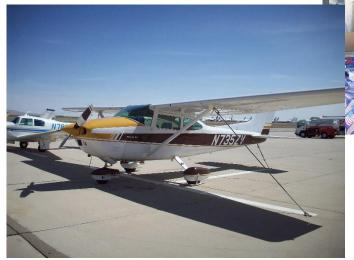
Roy Martin brought his 1964 Cessna 206 out again for display. It has a Continental IO-520 fuel injected engine with six opposing cylinders, developing 300 horsepower.
